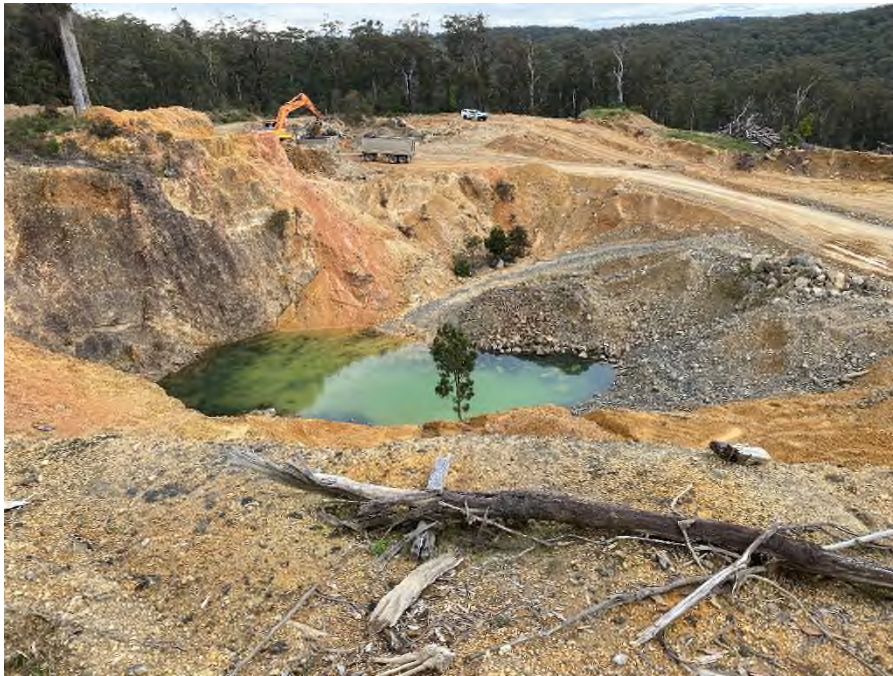
Photograph 2 , shows the existing quarry pit, viewed towards the northwest. The water in the base of the pit is visible. The area where material is currently being excavated from can be seen where the excavator is working in the background.
